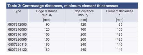
In order to ensure a save load transmission by the installed Fixing socket the basic conditions given in Table 2 must be paid attention to. If a higher concrete cover is required, the dimensions of the concrete element must be adapted accordingly.
